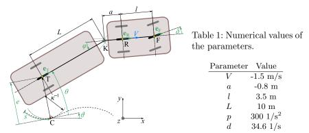
Fig. 1: Single-track kinematic model of the truck–semitrailer.
